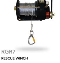
The RGR7 has a working length of 15m and 50m and is fitted with an up/down clutch-locking mechanism. Manufactured from steel, this winch has a 50cm diameter handle turn. One full handle turn will release approximately 48mm of cable to allow the worker to ascend / descend to safety. It can be fitted to the RGR1 tripod for use in confined space access when ladders or foot irons are not available.
